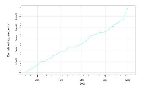
Figure 3: Cumulated squared prediction errors for the Tunø off-shore wind farm
