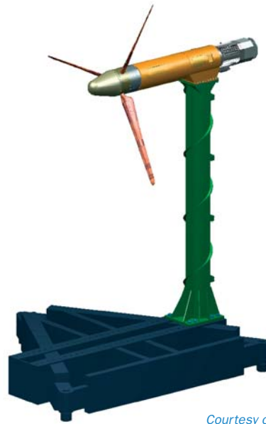
MEXICO: CAD drawing of model of wind turbine in the wind tunnel.
